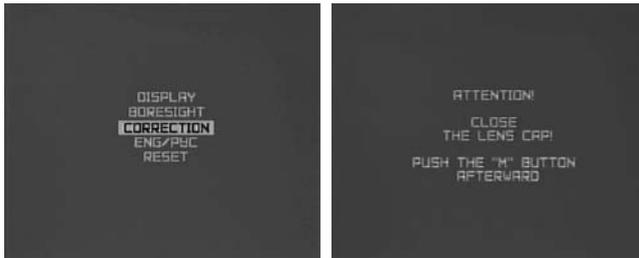
Make sure the lens cap is closed and press and hold (more than 2 sec) button M. The Correction menu appears on the screen.
