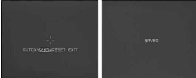
**To cancel** the dead pixels removal press and hold button M for more than 2 sec with the option “Reset” selected. The display shows the confirmation request.
