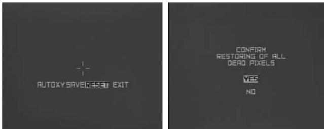
**To confirm** with buttons A or B select option “Yes” and press and hold button M for more than 5 sec. to cancel the correction.
