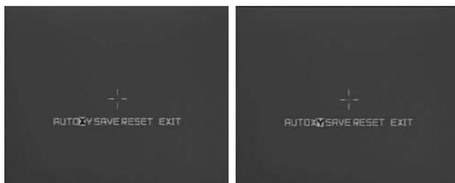
**To save** the dead pixel correction results press and hold button M for more than 2 sec with the option «Save» selected. The display shows the message confirming the successful saving.
