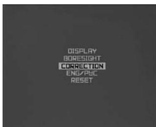
**To remove manually** the dead pixels press shortly button M to switch between X and Y. With X selected buttons A and B move the cursor horizontally, and with Y selected – vertically. Align the cursor center with the dead pixel and press and hold button M for more than 2 sec.
