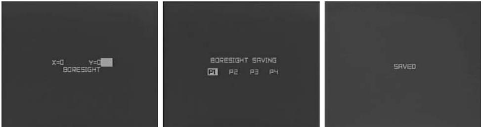
If the zeroing results are satisfactory, save the profile by pressing and holding (more than 2 sec.) button M, and the window of the profile selection will open.
